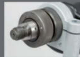
adjustment ring for soft percussion
