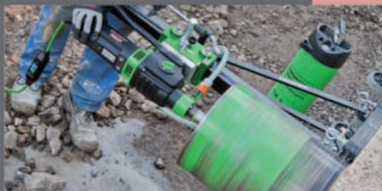
BST 352 V: mounted carriage on 4 special balls
