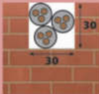
slitting of cable channels
